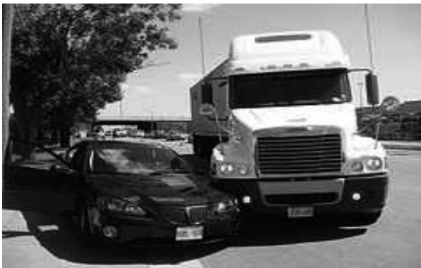
Fig 16: The driver of this car tried to pass the truck on the right side as the truck driver was preparing to make a right turn.
